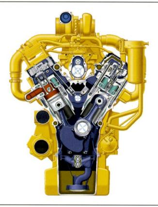
Cat 3412E engine, with the hydraulically actuated, electronically controlled unit injector fuel system (HEUI), offers superior lugging performance, fuel efficiency and reliability. The 12-cylinder engine is turbocharged with a high displacement-to-horsepower ratio. This large displacement produces better lugging capability, lower internal stresses and longer component life.
