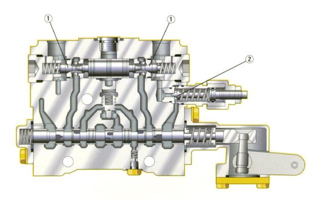
Power on demand. Normally, the variable displacement pump idles at near-zero output. When it senses a load requirement, the pump supplies flow and pressure to match the demand. The result is less hydraulic system heat and lower horsepower consumption.
