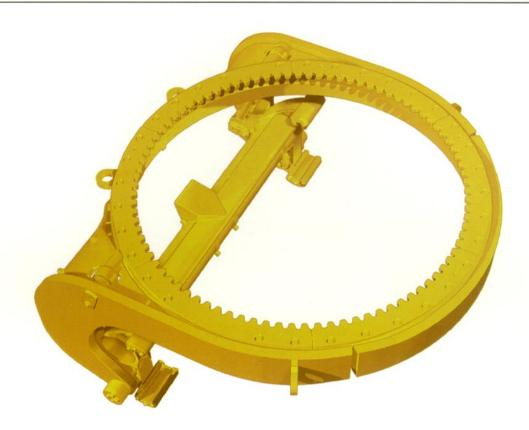
Rugged construction. The drawbar features an A-frame, box-section design for high strength. The bottom is machined to provide accurate adjustment and precise blading. A one-piece forged circle is built to stand up to high stress loads. To resist wear, teeth are flame-hardened in the front section. For maximum support, the circle is secured to the drawbar by eight support shoes with replaceable strips.
